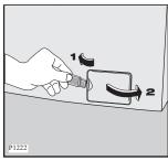
place a bowl with a small edge close to the pump to collect any spillage
